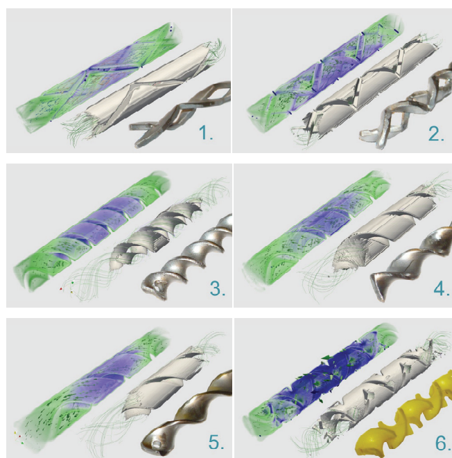
Figure 3. CFD pictures generated with ParaView [8] static mixers: 1) zigzag h/d = 2 , 2) zigzag h/d = 1.2 , 3) spiral h/d = 1 , 4) spiral h/d = 1.5 , 5) spiral h/d = 2 , 6) Kenics® static mixer.
