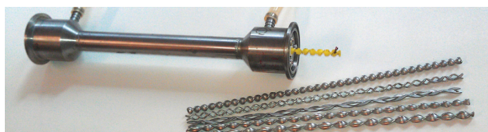
Figure 2. Kenics® static mixer in membrane module (left), 5 new turbulence promoters (right).
