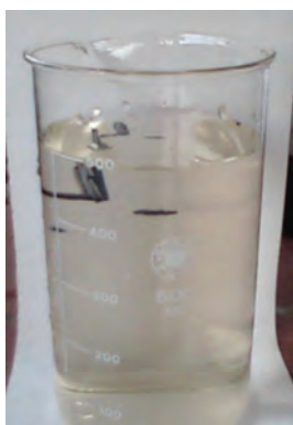
Slika 5. Izgled uzorka otpadne vode pre tretmana feratom(VI). Figure 5. Physical samples of wastewater before treatment by ferrate(VI).
