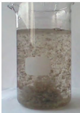
Slika 6. Izgled uzorka otpadne vode po dodatku ferata(VI), koagulacija i obrazovanje flokula. Figure 6. Physical samples of wastewater by addition of ferrate(VI), coagulation and formation of flocs.
