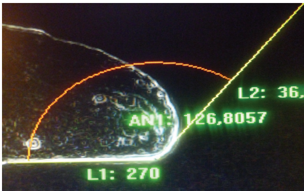
Figure 6. Analytical determination of contact angle for alloy Sn–12Zn–8Sb and Cu substrate (superheat temperature, 100 °C above liquidus temperature).
