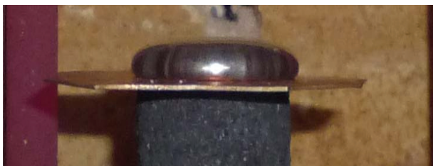
Figure 5. Formed alloy Sn–12Zn–8Sb drop on Cu substrate inside electrical resistance furnace (temperature superheat 100 °C above liquidus temperature).
