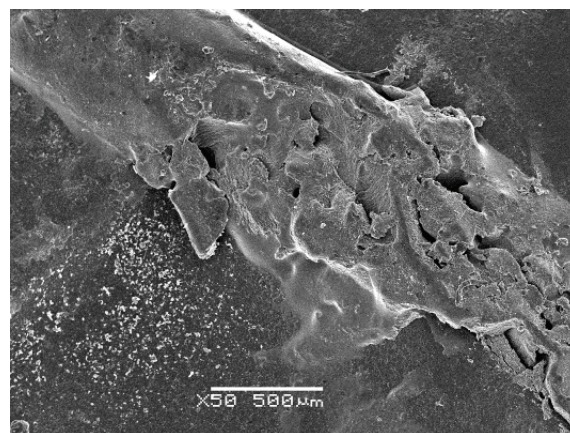
Figure 8. SEM micrograph – surface fragment of the composite cement after removal by prepolymerization (smaller magnification, 500 \times ).
