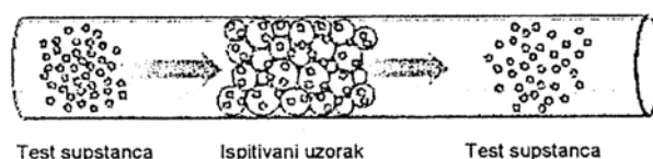
Slika 1. Princip rada gasne i inverzne gasne hromatografije [1]. Figure 1. The principle of gas chromatography and inverse gas chromatography [1].
