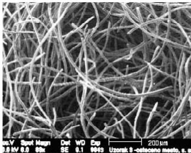
Figure 7. Microphotograph of the specimen 2CF after interaction with a ruby laser ( \Phi = 0.54 \text{ J}/\text{cm}^2 )
