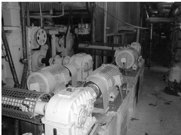
Slika 5. Pogonski motori i reduktori partije presa karton mašine Figure 5. Drive motors and recustors of the press of the paper machine
