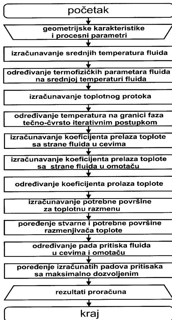
Slika 6. Blok dijagram programa za proveru performansi aparata Figure 6. Flow diagram for the rating calculations of heat exchangers
