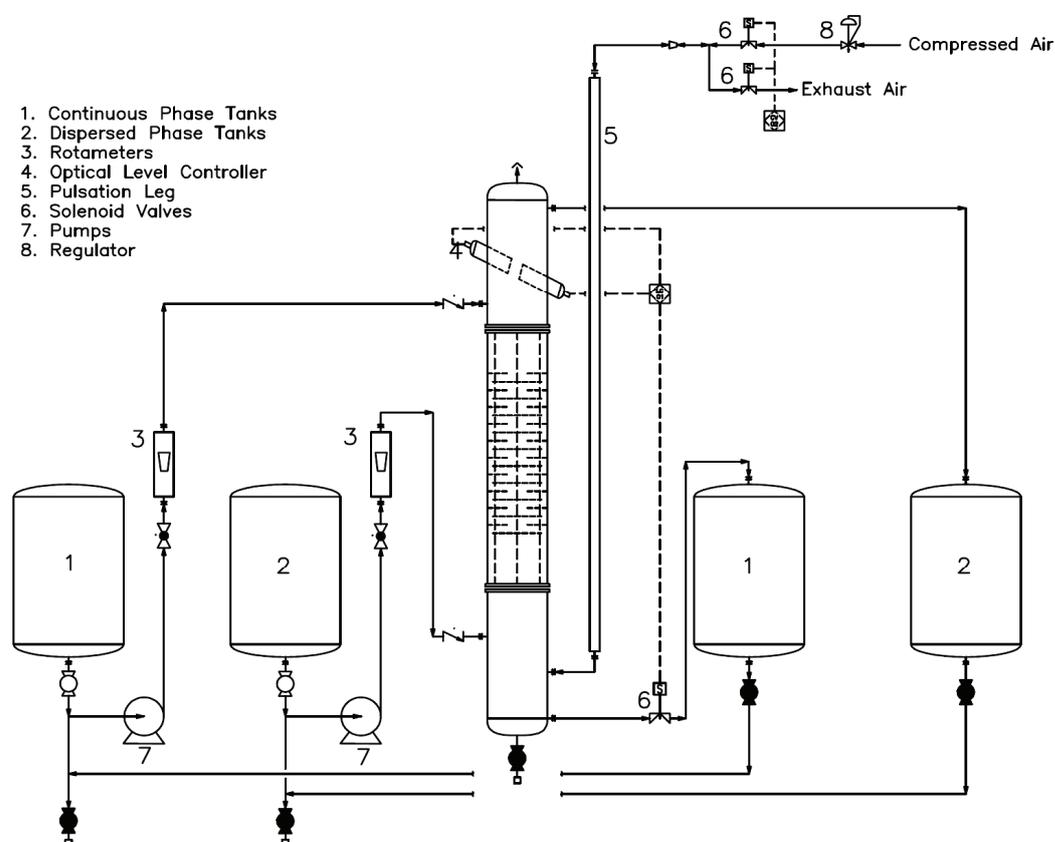
Figure 1. Schematic diagram of the pulsed disc and doughnut column.
