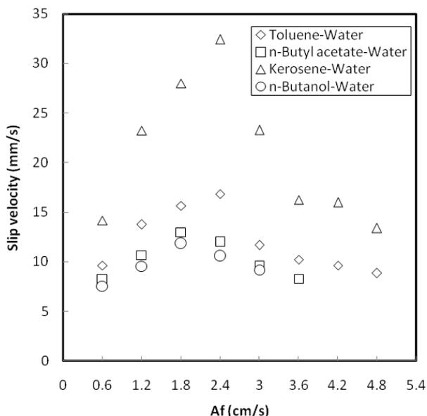
Figure 3. Effect of pulsation intensity on slip velocity ( $V_c = V_d = 1.132$  mm/s).
