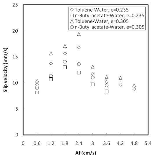
Figure 6. Effect of fractional free area on slip velocity ( $V_c = V_d = 1.132$  mm/s).
