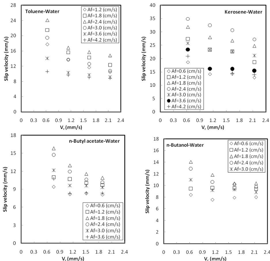
Figure 5. Effect of continuous phase velocity on slip velocity ( $V_d = 1.132 \text{ mm/s}$ ).
