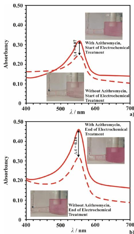
Fig. 3. UV-Vis spectra and photographs of the bulk electrolyte ( $0.05 \text{ M NaHCO}_3$ ) in a electrochemical cell in the absence and in the presence of  $0.60 \text{ mg cm}^{-3}$  of azithromycin dehydrate a) before and b) after four hours of holding the potential at  $-1.2 \text{ V}$  vs. SCE.
